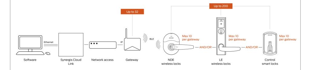
Gateway communication range up to 30' in typical building environments; a detailed site survey is recommended.
