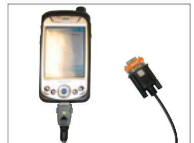
Serial Communication with Null Modem (PIMWA-CV) (BM-150)
