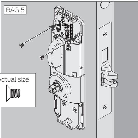
9d Secure bottom with two (2) screws.
