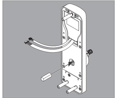
8b Route cables and posts through holes as shown. Push assembly against door and hold.
