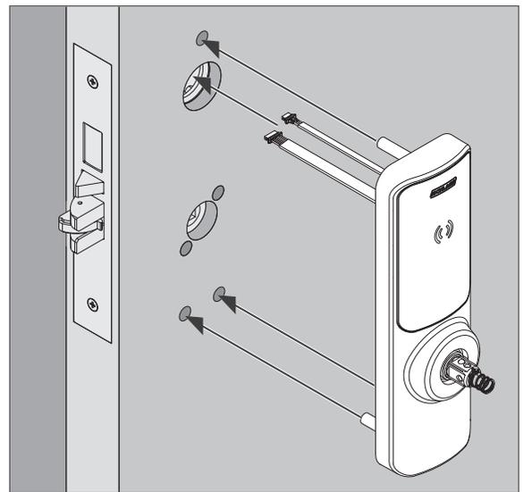
8c Route cables through gasket on interior plate. Install three (3) screws.
